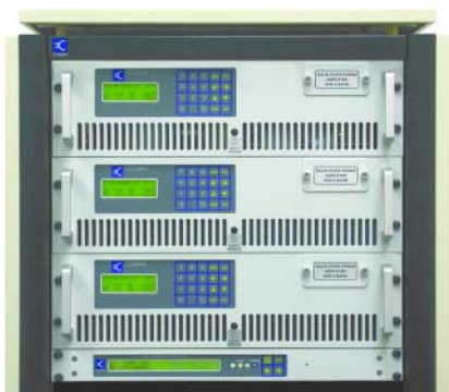
Front view of 1:2 SSPA redundancy system
